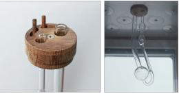
Viscometer tube holders
